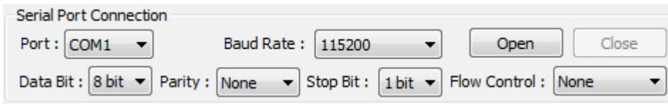
Make sure to select the correct COM port and click the open button, the Intelimax LITE GUI will connect to the modem via the selected COM port.
